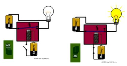
A relay is an electrically operated switch. It works on the principle of a magnet attracting iron when a current is flowing, closing the switch and creating a complete circuit and releasing it when the current is no longer flowing therefore opening the switch
