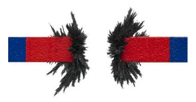
Like poles will repel each other. e.g. north and north. Unlike poles will attract each other. e.g. north and south A magnet is an object that has a magnetic field around it and attracts objects made of iron. A magnetic field is a region around a magnet where iron objects have a force on them and can be made to move.
