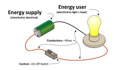
There is a need for a complete circuit when making use of electricity. A circuit must be closed for the charge to flow and produce a current.
