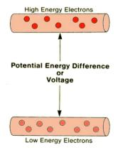
An electric current will not flow through a circuit unless there is a source of energy like a battery or mains electricity to push the electric charges along through the wire.
