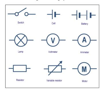
Circuit symbols are used to represent components of an electrical circuit. These symbols can be used universally by electricians and scientists regardless of their different languages, to show how different circuits are arranged.
