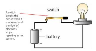
A circuit is made up of electrical components connected together so charge, carried by electrons, moves through the components. A battery or a cell is an energy supply. It supplies energy to the charges. The charges then move around the circuit carrying the energy. When the charges get to a user (or component) of the circuit e.g. a lamp, they have to work to get through the part. The energy is changed into another type of energy (e.g. heat, light, sound, movement).
