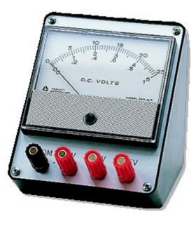
The unit is the volt, V. We can measure the energy of electric charges in a circuit before they enter a bulb and after they leave it by putting a voltmeter in parallel across the bulb.
