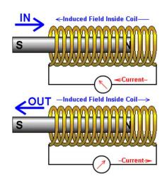
Electrical currents moving around a magnet can produce an electromagnet
