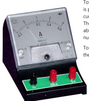
To measure current we need a charge counter which is "in" or is part of the circuit. We can measure the amount of electric current flowing in a circuit with a device called an ammeter. The unit of electric current is the Amp - which is often abbreviated to the letter A, especially if it comes after a number. So, for example, 3 Amps can also be written 3A.
