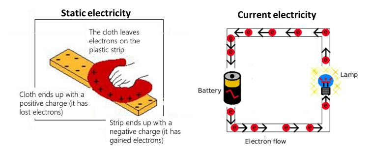
There are two types of electricity. Static electricity involves charge that is built up on insulators, usually by friction and when there is a large force acting on the charge, the charge will suddenly move. Current electricity involves the movement of charge through a conductor and it flows continuously if a pathway is formed.
