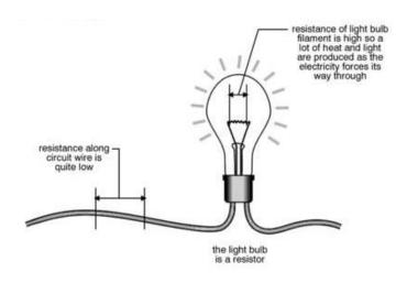
Parts of a circuit which offer high resistance transform a greater amount of electrical energy into light and heat energy. This is why the high resistance, very thin wire of a filament light bulb glows hot and bright while the lower resistance thicker wire providing the current to the bulb stays cooler.
