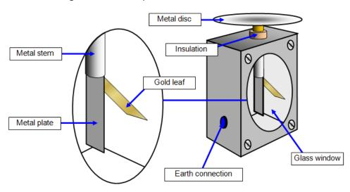
An electroscope can detect charge by induction or contact. A charged object is placed on or near the metal disc. A negatively charged object will repel negative charge in the insulated electroscope. The negative charge will travel down to the gold leaf and metal plate (some electroscopes have two gold leaves). The negatively charged leaf/plate will then repel each other and move apart. The more they more apart the more the charge held in the original object
