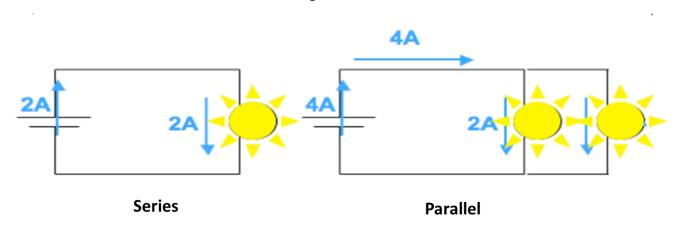
Predictions can be made about the current (amps) in both the series and parallel circuits using the rules. In a series circuit if one component reads 2A then all components will read the same. In a Parallel circuit the current reading leaving the power supply must be divided between branches.
