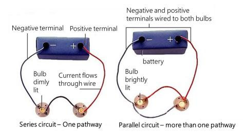
In a series circuit, the charge moves along one path only. The electrical current flows through one component then the next – more lamps added in series cause their brightness to decrease.
