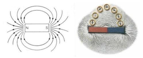
A magnet has a magnetic force field around it. When another magnet or an iron object enters the field, it experiences a force as either a push or a pull. Field patterns produced by bar magnets can be visualized using iron filings. This is the magnetic field. The field lines move out from the N end of a magnet and into the S end.
