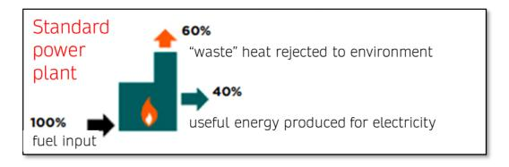
For example, from the diagram above of a traditional power plant more energy is waste than useful. Newer designed power plants are developing ways to reuse most of the waste energy to generate further electricity.[
