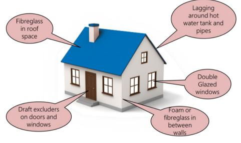
It is important to reduce the loss of heat from our homes. This is done by increasing the insulation of our homes using the methods shown in the diagram above.
