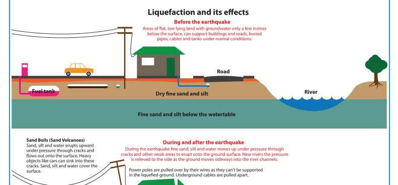
Fine sand and silt liquefies, and waterpressure increases
