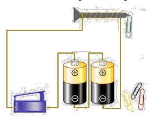
A magnetic field can be made stronger with a coil of conductive wire wrapped around it and an electric current flowing through the wire. This is called an **electromagnet**. An electromagnet can be made stronger by increasing the number of turns (how many times the wire is wound) and by increasing the current. A coil of wire is called a solenoid.
