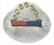
This is the **magnetic field**. The field lines move out from the N end of a magnet and into the S end. Compasses, which contain a movable magnet, can also be used to show magnetic fields. The needles will align in the direction of the field.
