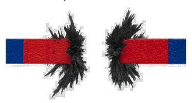
Like poles will repel each other. e.g. north and north. Unlike poles will attract each other. e.g. north and south A magnet is an object that has a magnetic field around it and attracts objects made of iron. A magnetic field is a region around a magnet where iron objects have a force on them and can be made to move.
