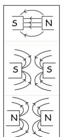
A strong field is produced between **unlike poles**, moving in the direction between North to South., shown by arrows
