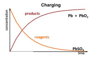
During **charging** of a battery the products from the discharging are now the reactants. In the case of the lead-acid battery the amount of PbSO $_4$  will be decreased and deposited back on the anode and cathode as Pb and PbO $_2$  respectively. Substances will now be in sufficient supply to begin discharging the battery once more.
