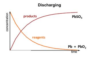
During **discharge** of a battery the amount of reactants (both the oxidant and reductant) will be decreased and the products formed increased. In the case of the lead-acid battery the Pb and  $PbO_2$  will be decreased (the anode and cathode respectively) and the solid  $PbSO_4$  will increase. Without enough reactants the Redox reaction will stop and the battery will stop producing voltage and become 'flat'
