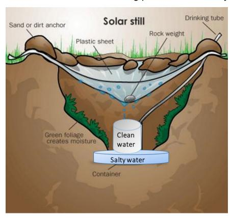
With a few pieces of equipment, a solar sill can be made to produce clean drinking water.
