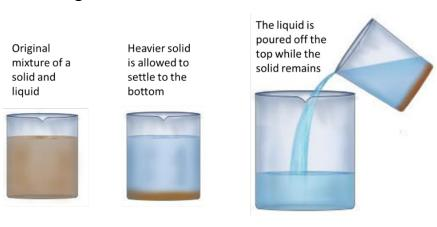
Decanting is simply pouring off a liquid without losing any of the denser substance (usually an insoluble solid) in the bottom of the container. Decanting separates a heavier substance from a lighter one. Chemists are most often after the substance at the BOTTOM of the container.
