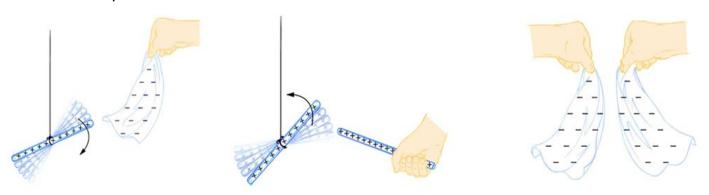
There are only two types of charge, which we call positive and negative. Like charges repel, unlike charges attract, and there are electric forces between charges. Both positive and negative charges exist in neutral objects, but they can be separated by rubbing one object with another. For objects (large enough to be visible), negatively charged means an excess of electrons and positively charged means a depletion of electrons (that have been removed). Charge is measured in coulombs (C)
