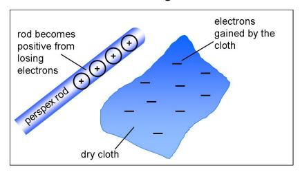
No charge is actually created or destroyed when charges are separated. Instead, existing charges are moved about. In all situations the total amount of charge is always constant. This universally obeyed law of nature is called the **law of conservation of charge**.
