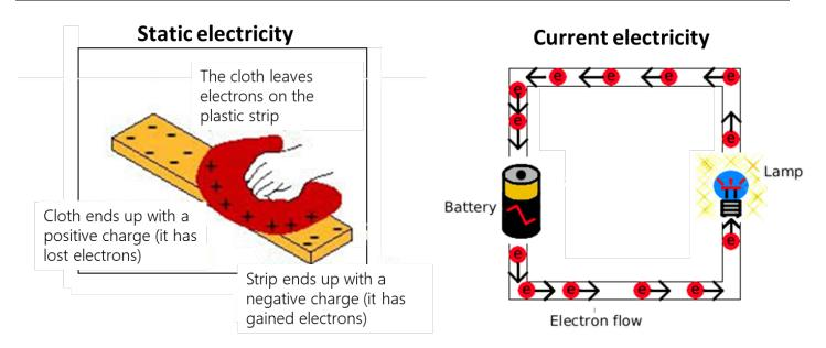
There are two types of electricity. **Static electricity** involves charge that is built up on insulators, usually by friction, and when there is a large force acting on the charge, the charge will suddenly move. **Current electricity** involves the movement of charge through a conductor and it flows continuously if a pathway is formed. Electric charge produced by friction is the same charge which, moving around a circuit, produces an electric current
