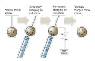
Objects can also be **charged by induction**. When a negatively charged object is held close to another object but not touching then the negative electrons are repelled and move away (if a path is created which "earths" the object) and the non-moving protons cause the object to be positively charged.
