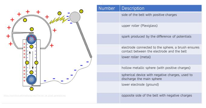
**3b.** Why does a spark occur when the spherical device is held close to the van der Graaf generator? In your explanation use the terms: *imbalance, charge, discharge, positive, negative.*
