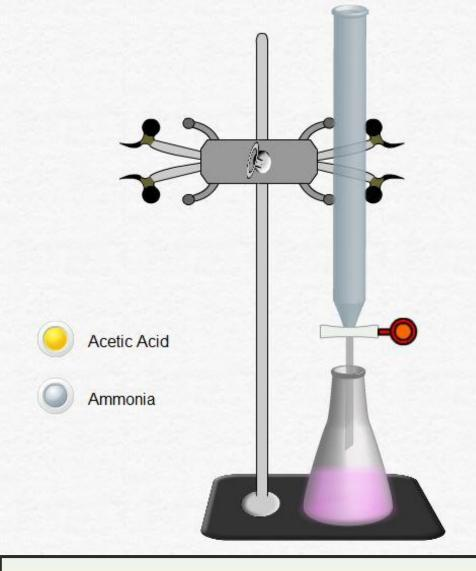
Titration of CH<sub>3</sub>COOH(aq) [V = 40.0 mL, C = 0.200 mol/L] with NaOH(aq) [C = 0.200 mol/L] using phenolphthalein indicator.
